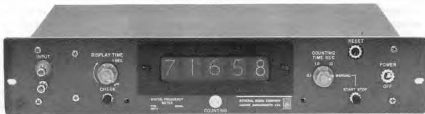
Figure 1. The Type 1150-A Digital Frequency Meter. Encased in General Radio's multi-purpose cabinet, 4 the instrument is readily mounted in a rack or adapted to table-top use with end frames. The panel is 3½ inches high. The controls and fittings are simple and clearly marked. Frequencies between 10 cps and 220 kc can be counted over preselected time intervals from 0.1 to 10 seconds. Display times can be continuously adjusted from 0.5 to 5 seconds and ∞.
